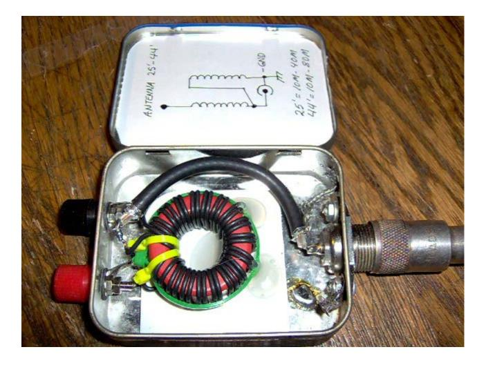
Here's a picture of my UNUN showing just how it is layed out and you can even see the schematic for it pasted inside the lid of the box. The antenna wire connects to the red binding post, and the counterpoise wire connects to the black binding post. Try to get the antenna wire up with as much of it vertical as possible and the rest of it horizontal in an inverted L fashion, or you can use it as a sloper just as I mentioned above.
