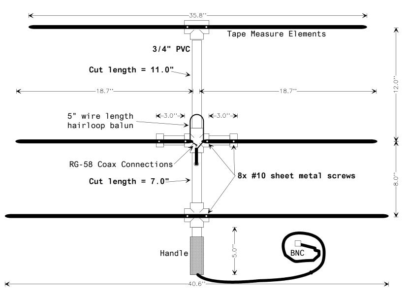
2m Tape Measure Sniffing Antenna (~78 db F/B ~7.5 dbi Gain on 146.565) original design by WB2HOL - tweeked & modified by N6JSX/8, 2004
